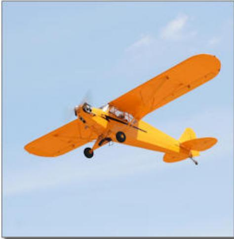
"You are correct; the use of power on the approach depends upon the type of aircraft. Some of the heavier airplanes develop rather high sink rates with no power on the approach. In light airplanes such as a J-3 Cubs and Champs, power off approaches are desired.
